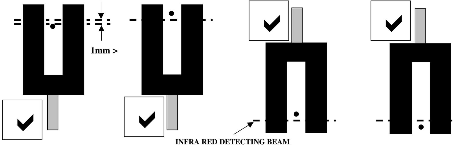
POSITIONING THE YARN CLOSE, OR IN THE INFRA RED DETECTING BEAM WILL RESULT IN FALSE COUNTS.
