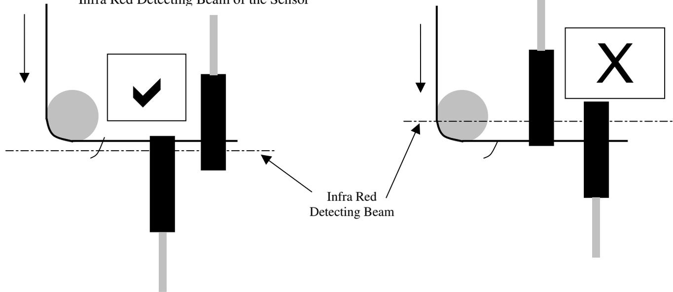
POSITION OF THE BFD SENSOR TO THE YARN TOP MUST NOT BE CLOSER THAN 1mm FROM THE INFRA RED DETECTING BEAM
