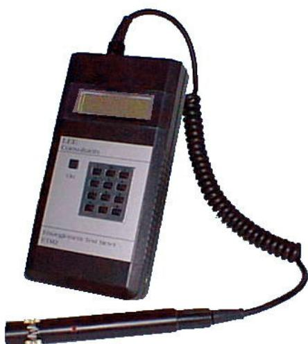
The instrument is capable of measuring entanglement points on textured and flat yarn at speeds up to 5000 M/min. Different amplification levels can be selected to suit various signal levels generated by a wide range of yarns and entanglement points. This makes the ETM3 suitable for all types of air jet application on draw texturing, draw twisting, draw winding, POY spinning and draw warping.
